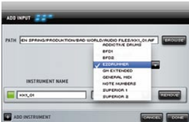
Assigning an internal sound device to later receive the generated MIDI events (in this case "EZdrummer" by TOONTRACK)
