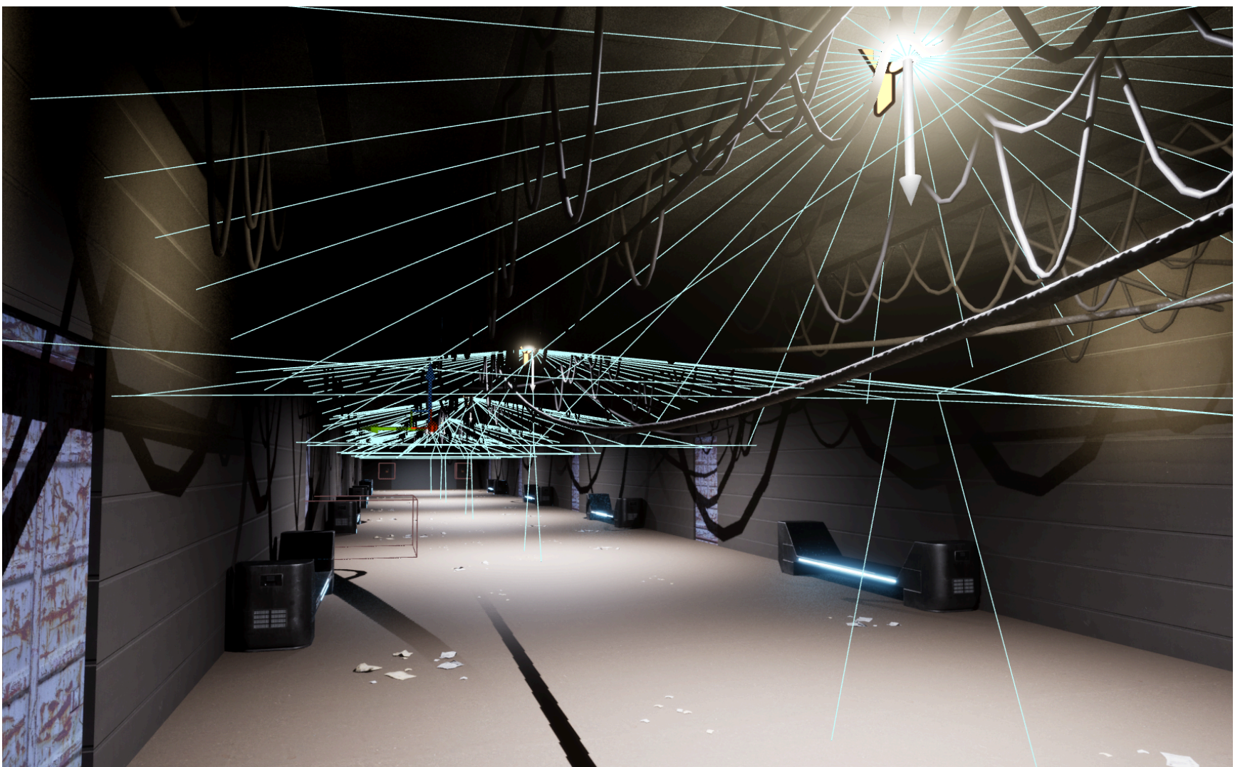
Similarly the hallway was lit using spotlights but with the outer core angle at 80 degrees.
